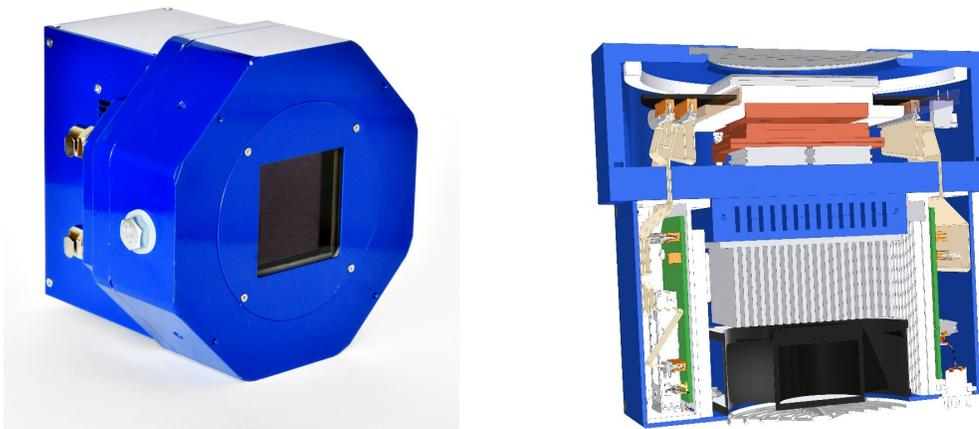
**Fig. 1.** Exterior view of the pCam6060 photodetecting system (left) and the design scheme of the pCam6060 vacuum chamber internal structure (right).
