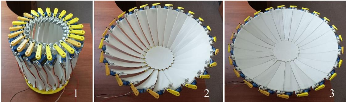
**Fig. 1.** The stages of deployment of the physical model: 1—mirror in the folded state, 2—partially opened mirror, 3—mirror in the opened state.
