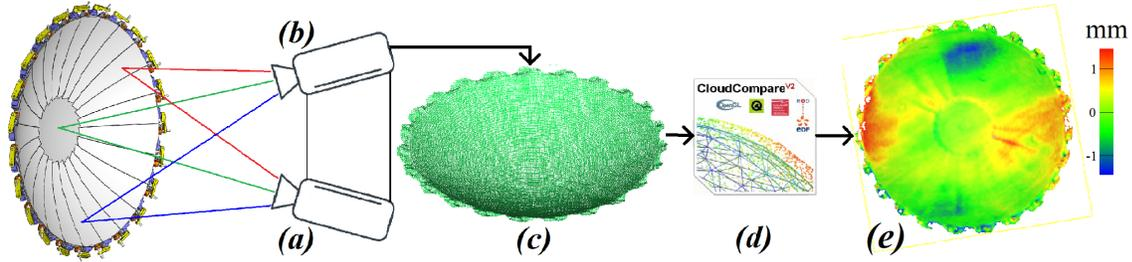
**Fig. 2.** The process of scanning and analyzing the mirror surface. (a, b)—3D scanner (the projection unit and registration unit, respectively); (c)—point field; (d)—CloudCompare; (e)—a result of the scanned data processing using CloudCompare.
